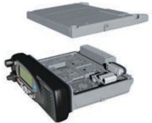
Inside the TM9155 mobile radio
